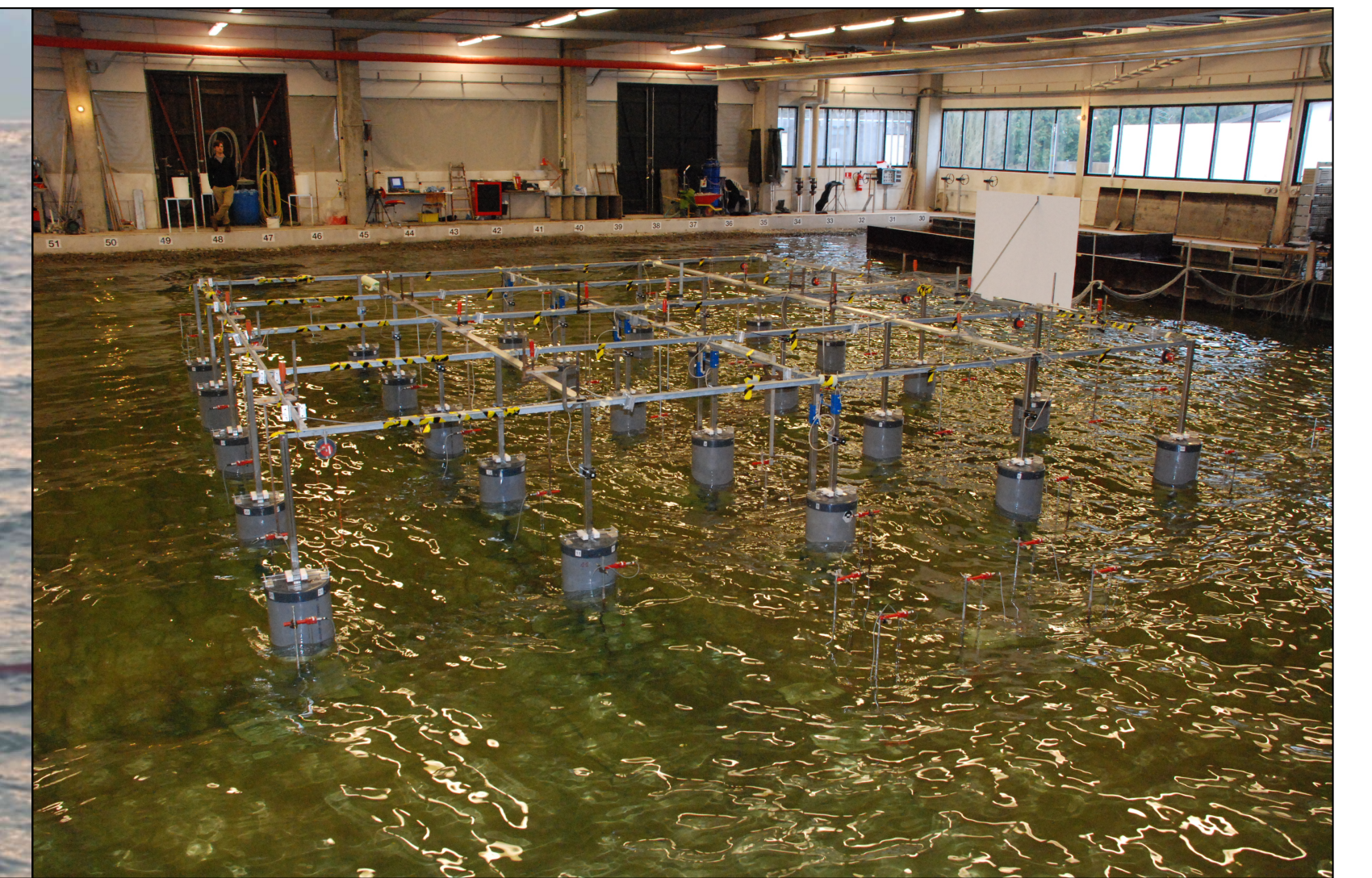
The WECwakes renewable energy project (led by UGent) modelled (in scale) an array of 25 wave energy converters to study the full 3D interactions of the devices with the wave field.
